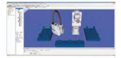
3D simulator for work cell layout and toolpath program testing
